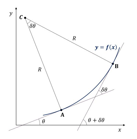
Gradient at A:  $\left(\frac{dy}{dx}\right)_{A} = \tan \theta$ Gradient at B:  $\left(\frac{dy}{dx}\right)_{B} = \tan(\theta + \delta\theta)$
