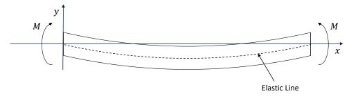
The elastic beam bending equation, which can be used to describe the bending moment, *M*, as a function of the radius of curvature, *R*, is:  $\frac{\sigma}{y} = \frac{M}{I} = \frac{E}{R}$  $\therefore \frac{1}{2} = \frac{M}{R}$
