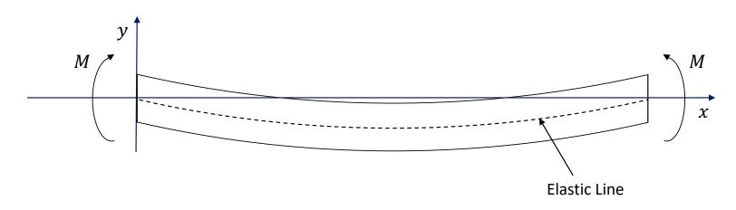
The transverse deflection of the elastic line is given by the co-ordinate, y, of any position along its length, x
